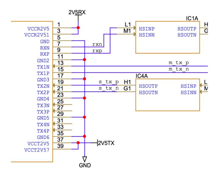
Table 9: VTRx+ module optical interface pinout.
